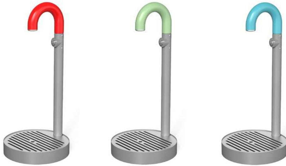
Drinking fountain composed of a steel tube structure, a chrome-plated brass tap with push button provided with a return spring and a circular tank. The latter is equipped with a drainage pipe with an overflow system and a removable drain for cleaning purposes.
