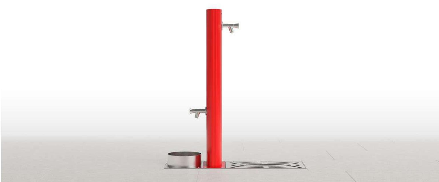
Fountain composed of an elliptical steel sheet structure and two chrome-plated brass push button taps: one with stainless steel bowl for animals, the other with a rectangular tank. The latter is equipped with two drainage pipes with an overflow system and a removable drain for cleaning purposes.
