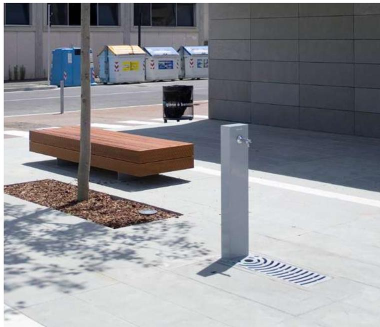
Collection of drinking fountains composed of a steel sheet structure, a chrome-plated brass tap with push button provided with a return spring and a rectangular tank. The latter is equipped with a drainage pipe with an overflow system and a removable drain to allow cleaning. The back of the tank is equipped with a slit for the connection of water supply. Three different models with rectangular, circular or elliptical.
